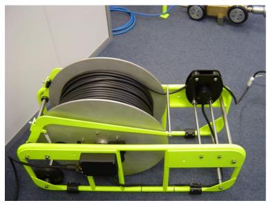
The 300m hand operated cable drum has a slip ring assembly and shaft encoder to monitor the amount of cable deployed. With the handle provided the drum can move easily on its wheels between deployments.
